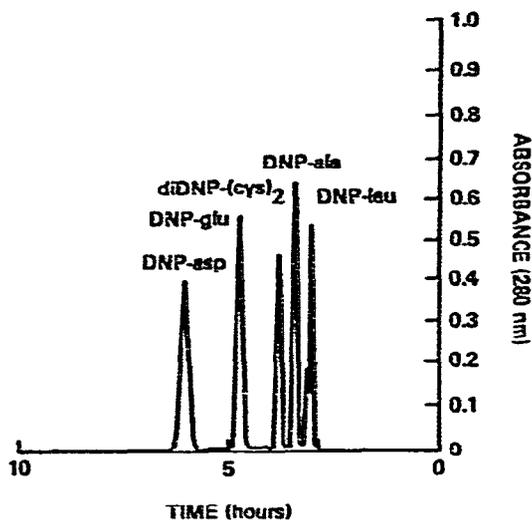
Fig. 2. Chromatograms of DNP-amino acids. A, Preparative-scale separations; solvent system: chloroform-acetic acid-0.1 M hydrochloric acid (2:2:1); sample volume: 10 ml; revolution: 400 rpm. B, Analytical-scale separations. Column: 0.55 mm I.D.; 24 ml capacity, pulley-side; solvent system as in A; sample volume: 50  $\mu$ l; revolution: 500 rpm; flow-rate: 6 ml/h; stationary phase: top, non-aqueous phase; bottom, aqueous phase.
