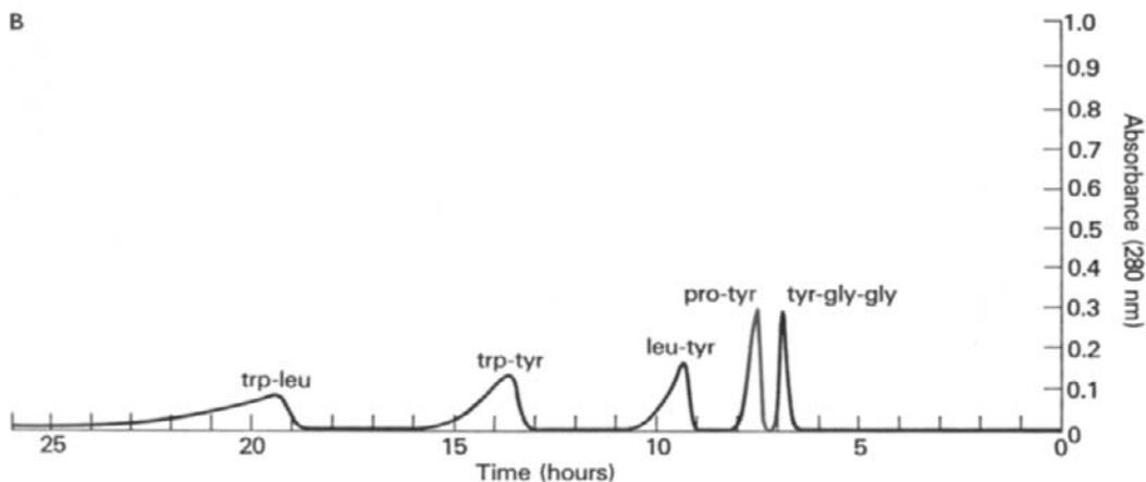
Fig. 3. Chromatograms of oligopeptides. A, Preparative-scale separations; solvent system: *n*-butanol-acetic acid-water (4:1:5); sample volume: 10 ml; revolution: 500 rpm. B, Analytical-scale separations. Column: 0.55 mm I.D.; 24 ml capacity, pulley-side; solvent system as in A; stationary phase: non-aqueous phase; sample volume: 50  $\mu$ l; revolution: 450 rpm; flow-rate: 2.4 ml/h.
